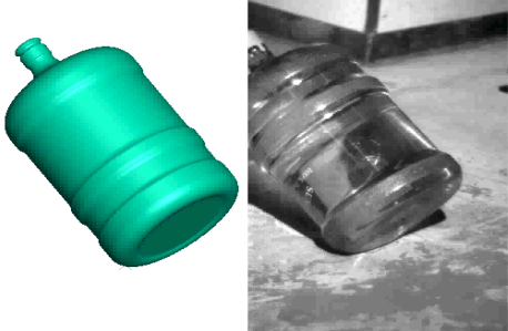
Water can drop test
