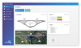
Dashboards to give quick overviews of the structure. With features such as: Images with live values, graphs with live data, tables with sensor values, and much more.
